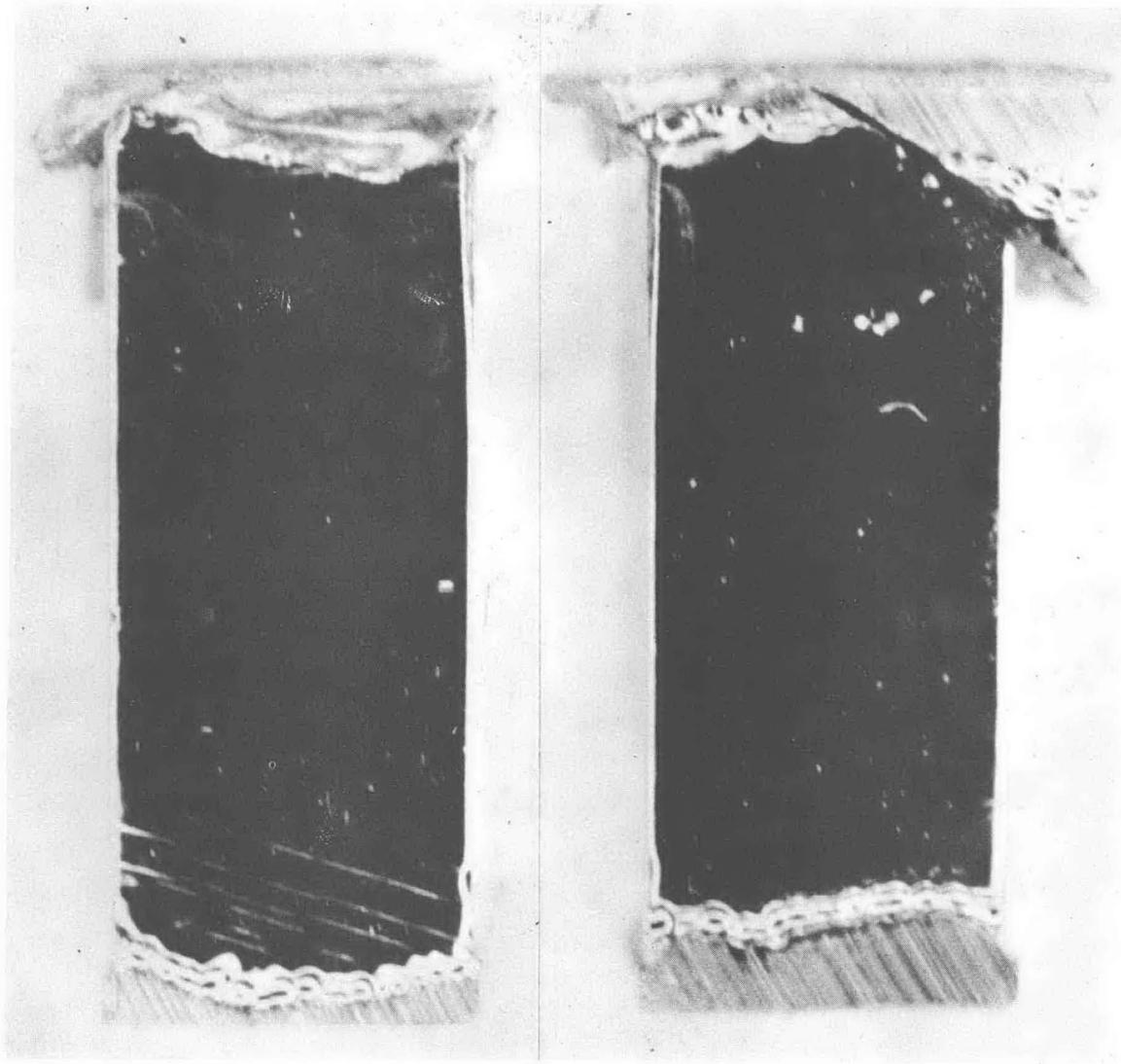
Fig. 8 - Macroscopic Photograph Showing {1120} and {1010} Lateral Surfaces of Crystal ISR-11 After c-axis Compression under Hydrostatic Pressure in the Range 238-255 ksi. Mag. 15X
